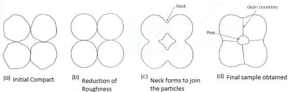
to cause the pellet to maintain a permanent structure. Figure 2 shows how sintering can be decomposed into four stages. It illustrates that the particles need not be spherical and how there is disruption at the grain boundaries causing them to disappear and reform.
