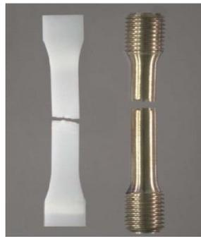
Figure 6: The figure shows typical tensile testing specimens. They have a thinner gage length between two gripping ends that are held by the testing machine. (Materials Evaluation and Engineering, Inc, 2009)
