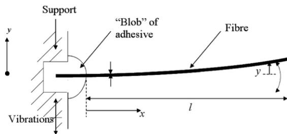
Figure 5: Fibres used by Perrin *et al.* were fixed into a support which was then vibrated. The free end of the fibre oscillated at varying displacements dependent upon frequency of vibration (Perrin, et al., 2007)
