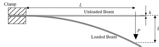
Figure 4: A simple sketch of a cantilever setup, unloaded and loaded beam (University of Cambridge, No date)
