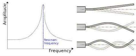
Figure 2: (right): Resonant nodes in a clamped bar, the top being the fundamental node and the ones below the subsequent nodes. (HyperPhysics, No date) (left): A graph that demonstrates how amplitude behaves near resonant frequencies (left) (Wikibooks, 2013).
