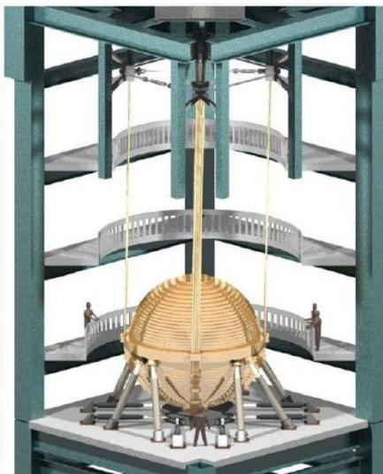
Figure 3: This image shows one of the tuned mass dampers in the Taipei 101, it is several stories high and the 660 metric ton weight sits upon hydraulic arms that damp the motion of the tower swaying. (probyte2u, 2011)
