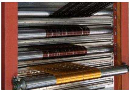
PAN fiber going through oxidation oven
