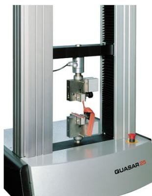
Figure 7: This figure shows an example of a universal testing machine. There is a fixed head at the bottom and an adjustable one above. This is used for applying tensions and stress's to samples. If plugged into correct software, it may generate a stress-strain curve. (Advanced Universal & Force Testing Technologies, No date)
